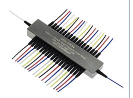
The MEMS Series N-bit (up to 16-bit) Photonic Time Delay digitally varies the delay time inside a fiber with exceptionally large range (maximum delay) and precision (bit). It selectively routes optical signals through N fiber loops whose lengths increase successively by a power of 2. Since each switching element allows the signal to either pass or bypass a fiber loop, a delay T may be inserted, which can take any value (in increments of  $\Delta T$ ) up to the maximum value T.
